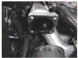
Looking at the photographs below, the restriction caused by the original valve can be seen clearly. Also notice the residual sludge build up left by the dirty exhaust gases!
