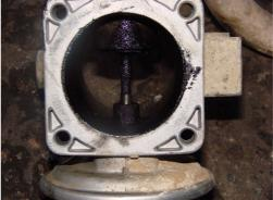
The exhaust blanking plate is simply attached to the exhaust manifold with the 2 Allen bolts. No gaskets are required for this, as both are machined flat surfaces, and will seal well. Just take care to nip the blanking plate up evenly on both sides.
