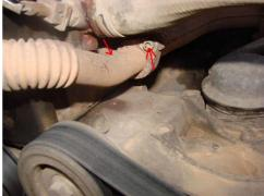
Remove the 4 x 8mm bolts, one of which is marked by the green arrow, holding the EGR valve to the inlet manifold. Remove the 2 x 8mm bolts, marked in blue, from the EGR re-circ pipe, where it fastens to the front of the cylinder head. (EU2 models only) Loosen the jubilee clip, marked by yellow arrow, and release the engine air intake hose from the EGR valve.
