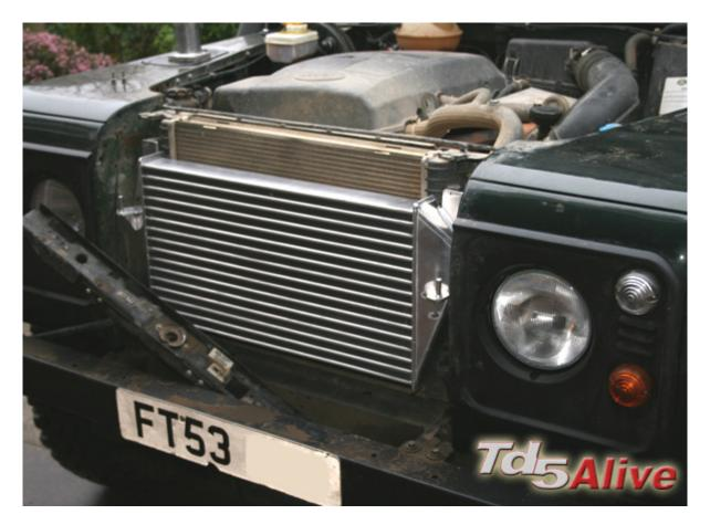
Your new intercooler should now sit snugly in place, so refit the intercooler hoses. Now you are ready to refit the two black plates over the intercooler front pegs and refit them to the wings using the 8mm bolts. Place the landing panel back into position and replace the four studs loosely. Fasten the brace bars back in place with the bolts. Note that the braces fit on the outside of the lower mounting points, Not the inside as there just isn't the room anymore!
