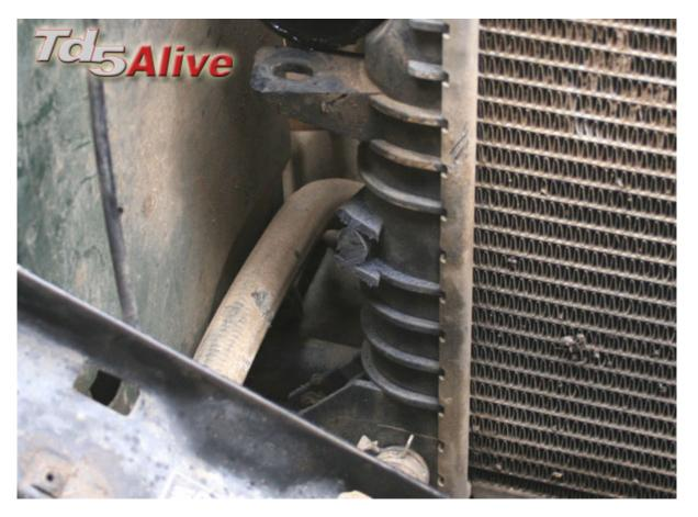
Once the original intercooler has been removed, you will need to cut a pair of plastic lugs off the coolant radiator. Using a junior hacksaw, remove these lugs so they no longer protrude from the radiator (Pictured above and below).
