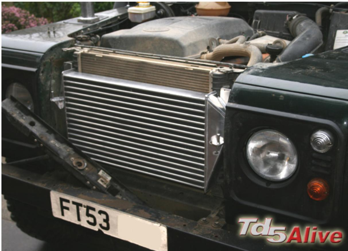
Your new intercooler should now sit snugly in place, so refit the intercooler hoses. Now you are ready to refit the two black plates over the intercooler front pegs and refit them to the wings using the 8mm bolts. Place the landing panel back into position and replace the four studs loosely. Fasten the brace bars back in place with the bolts. Note that the braces fit on the outside of the lower mounting points, Not the inside as there just isn't the room anymore!
