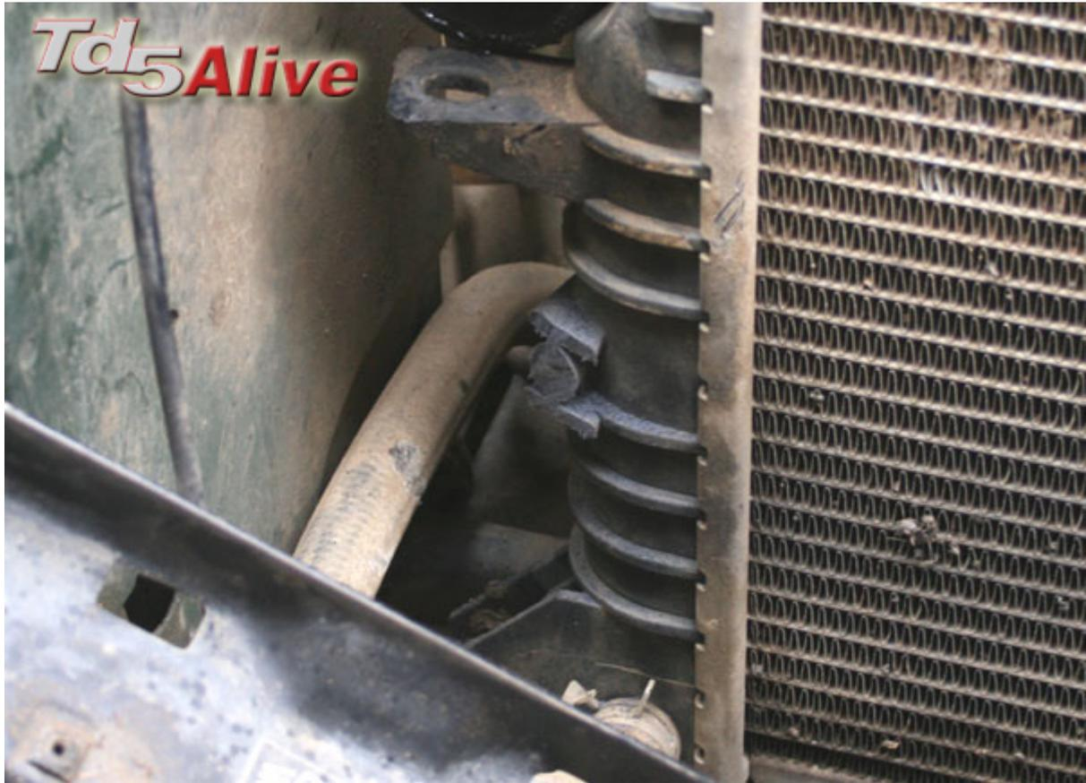
Once the original intercooler has been removed, you will need to cut a pair of plastic lugs off the coolant radiator. Using a junior hacksaw, remove these lugs so they no longer protrude from the radiator (Pictured above and below).
