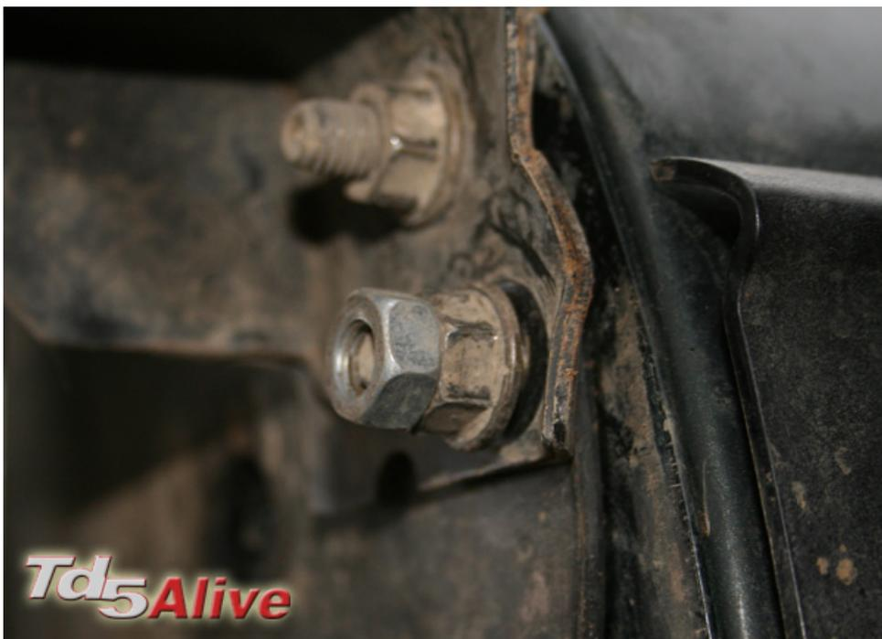
Undo the jubilee clips on both the intercooler inlet and outlet hoses, and pull them off. Also, the Intercooler is bolted onto the top of the radiator with two M8 (13mm) bolts, which you must remove. Once this is done, lift the intercooler off it's retaining holes on the coolant radiator, and pull it out completely.
